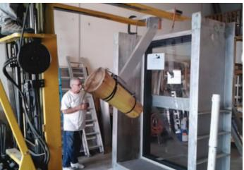
Flood debris testing of a proposed window assembly.
