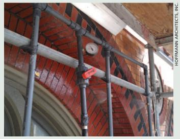
In the field: Spray-rack water test of a rehabilitated window.
