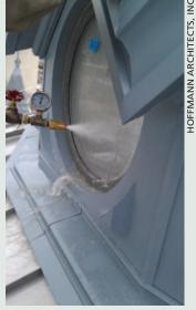
Water test of newly installed window.
