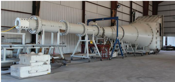
Shock-tube apparatus for blast-resistance window testing.
