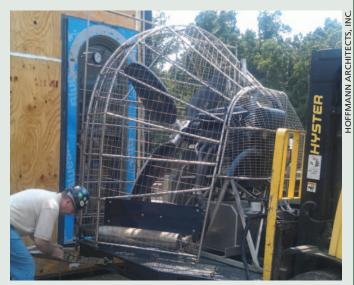
In the lab: Wind and water test preparation for a window PMU.
